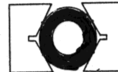
Four-point Contact with "Vee" Blocks
